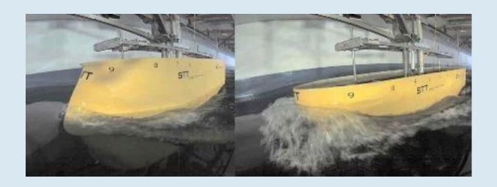
The **X-Bow** "pierces" the surf and disperses its energy to the sides of the **boat**. That means there's less of a rocking **motion**, which in turn reduces **motion sickness**
